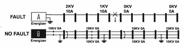
The voltage and current reading pictured above indicates there is **no** fault on your fence line.
